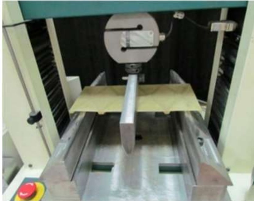
Fig. 4. IGSC specimen in the fixture of three-point bending test.
