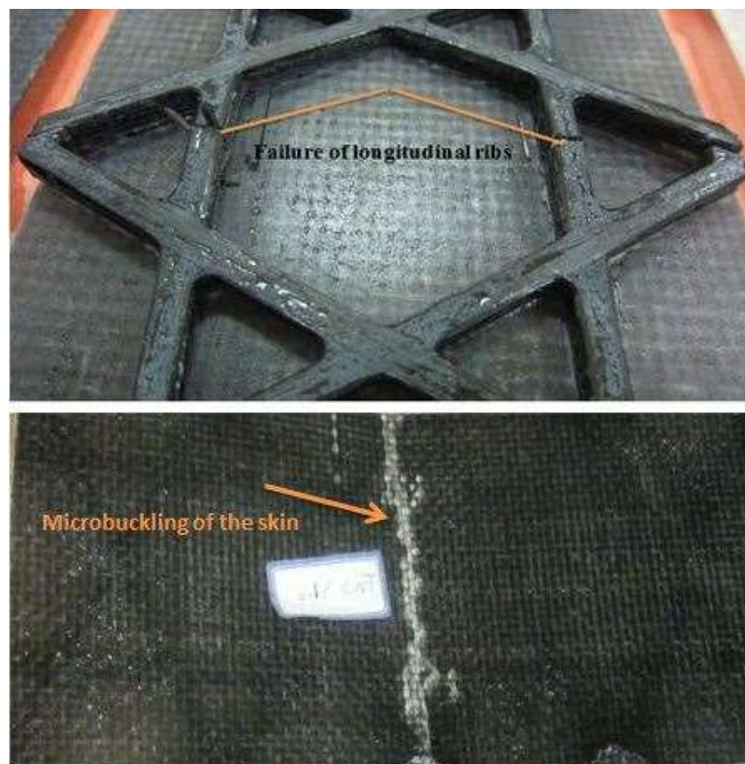
Figure 5. Various modes of failure in AGC panels under bending loading.
