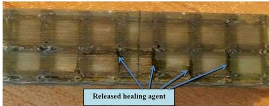
Figure 6. Filling the cracks with the released healing agent from the embedded network.
