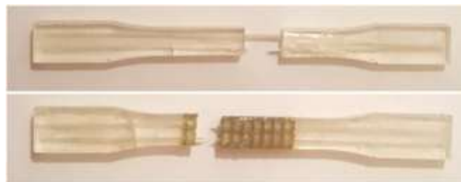
Figure 5. Tensile specimens with and without embedded network after failure.
