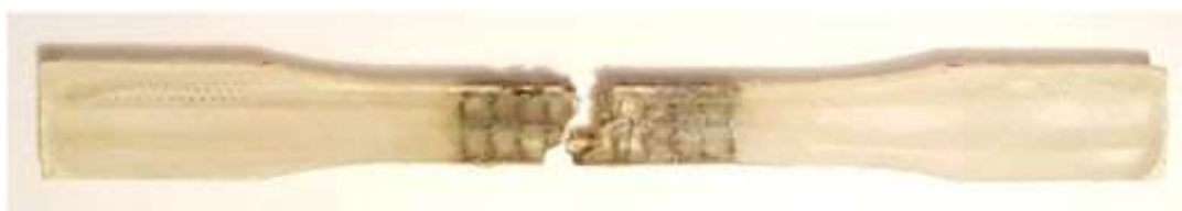
Figure 11. Self-healing specimen after creep test.
