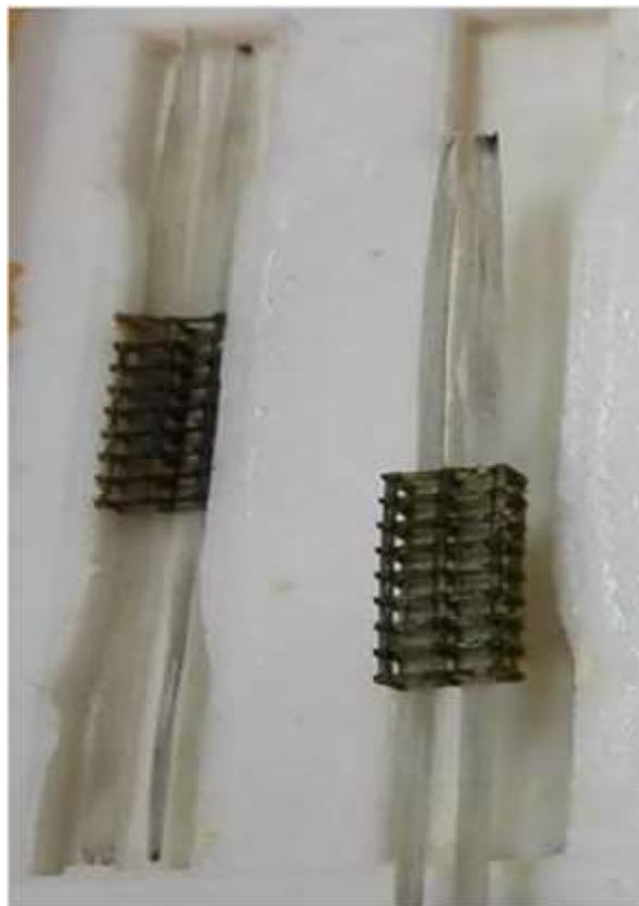
Figure 2. Embedding microvascular network and glass roving within the specimens.
