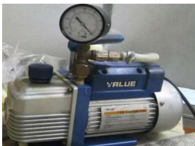
Figure 4. Vacuum pump for storing resin and hardener into the hollow glass fibers.
