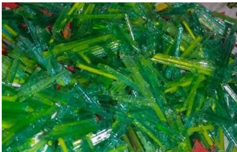
Figure 5. Short hollow glass fibers filled with resin or hardener.
