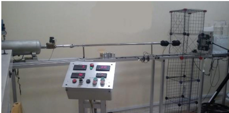
Figure 5. Gas gun high velocity impact tester.
