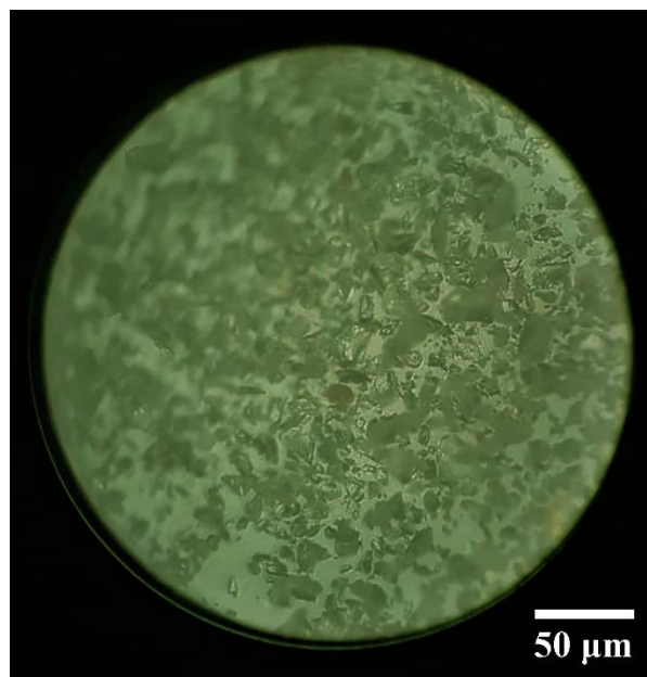
Fig. 1. Optical microscopy image of used SiO 2 particles in sandblasting.
