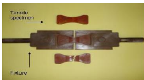
Fig. 2 - Closure of tensile strength in accordance with ASTM D 651.
