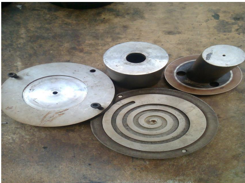
Fig. 1- Tools of flow test of composite samples for determination of B-stage optimum time.
