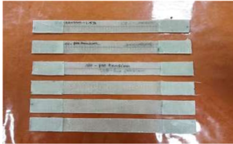
Fig. 2. SMAHC specimens for tensile test.
