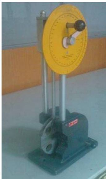
Figure 5- EMIC pendulum Charpy impact tester.
