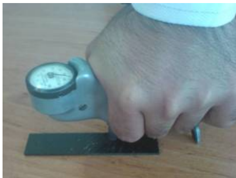
Figure 4- Impression made by Barcol impressor hardness tester.
