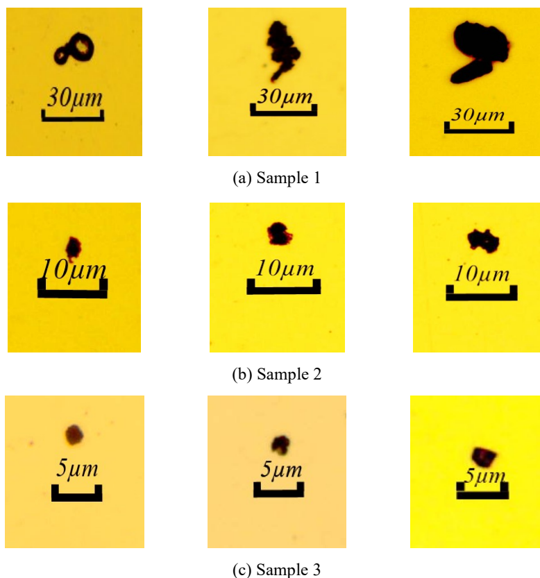
Fig. 2. Typical inclusions found in samples.
